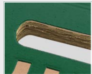
Cutting of mounting holes
