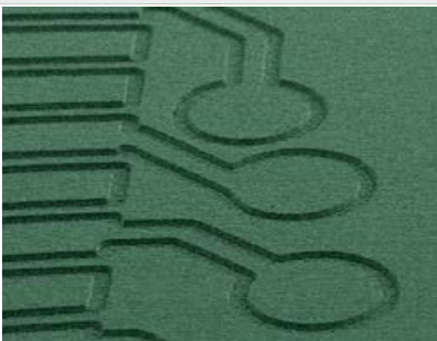
Direct light exposure of photoresists e.g. chemical tin for ultra fine structures
